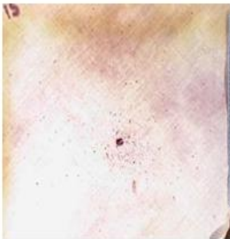
15 inch witness panel processed for lead residues
