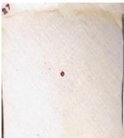
27 inch witness panel processed for lead residues
